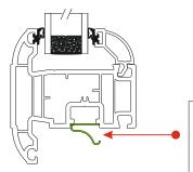
Fit a BC002 Sash Spring to the sash on the center line of the stay fixing
